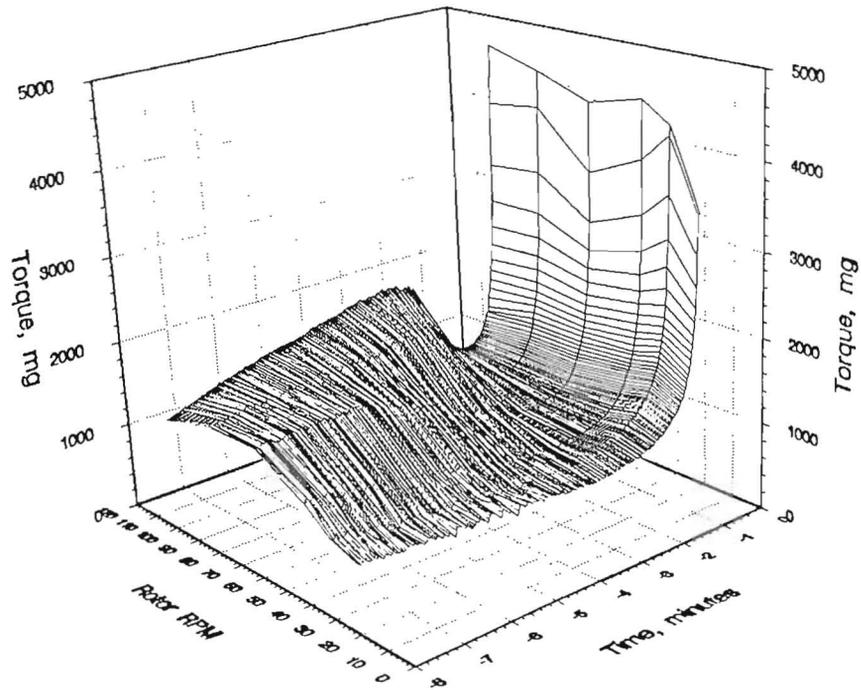
Fig. 9. Three-dimensional torque rheometry map: Variation in rotor rpm from 20 to 100.
