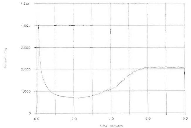
Fig. 13. Single run two-dimensional torque rheometry chart: highly filled PVC pipe compound, 60 rpm and 185°C.
