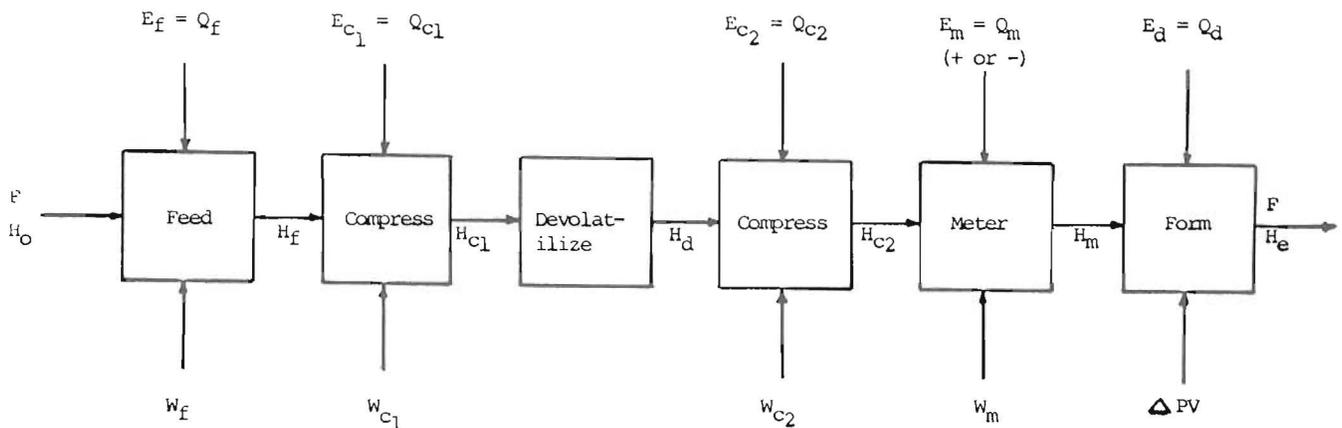
Fig. 3. Simple energy balance for a rigid PVC extruder.
