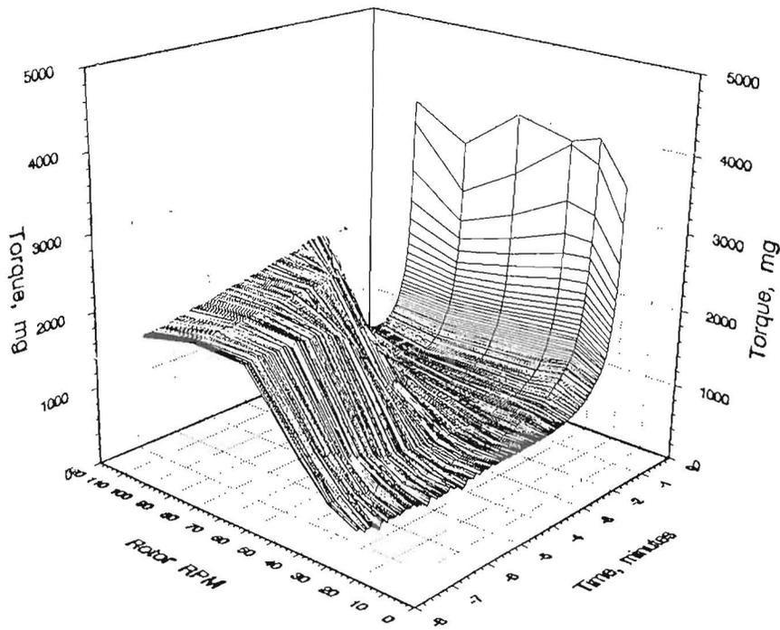
Fig. 14. Three-dimensional torque rheometry map: highly filled PVC pipe compound, variation in rotor rpm.
