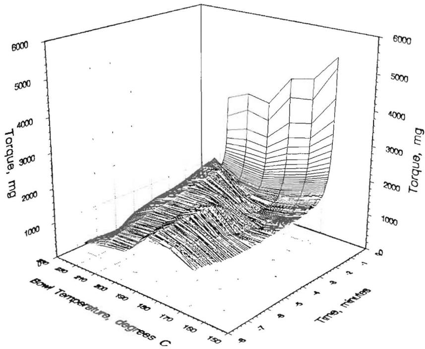
Fig. 10. Three-dimensional torque rheometry map: Variation in bowl temperature.
