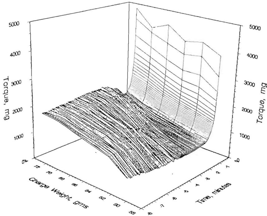
Fig. 11. Three-dimensional torque rheometry map: Variation in charge weight.
