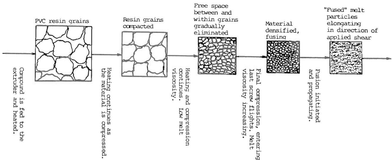
Fig. 4. Rigid PVC fusion mechanism in a twin screw extruder.
